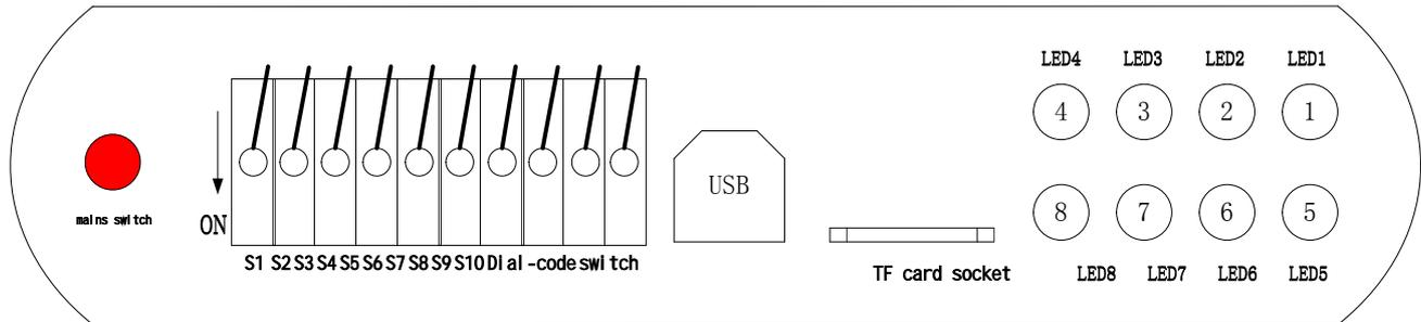
Figure 3 Schematic diagram of the front board interface of the CAN recorder
