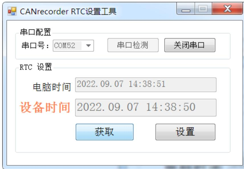
Figure 7. Configuring the equipment RTC time
