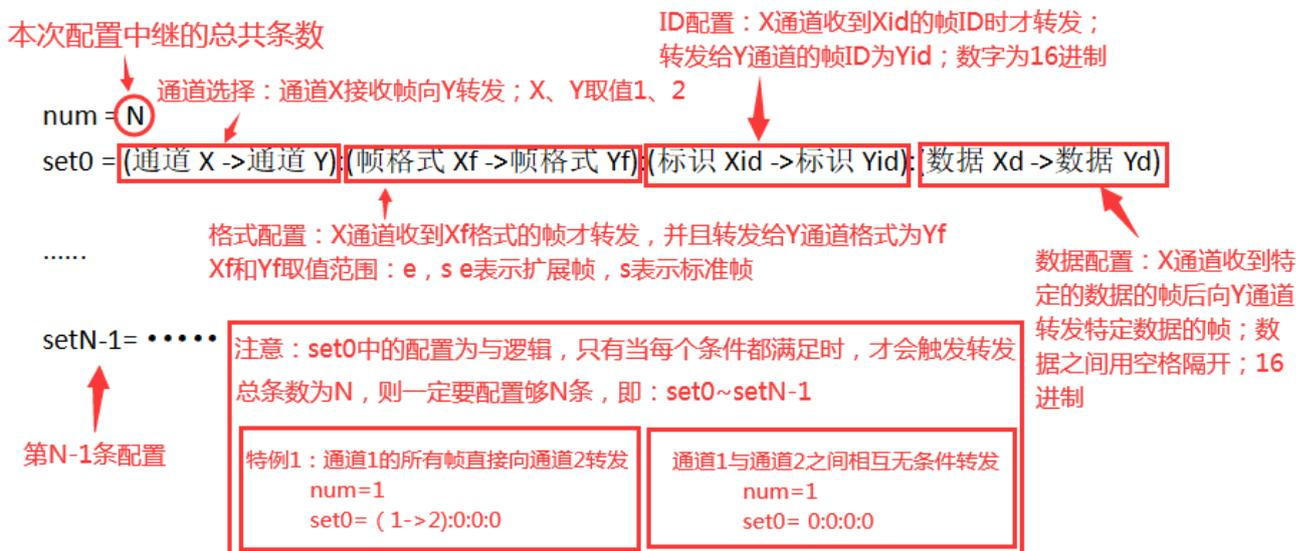
Figure 13. A schematic diagram of the relay function configuration
