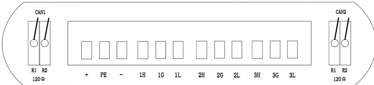
**Figure 4 Schematic diagram of the rear plate interface of the CAN recorder**
