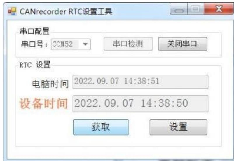
Figure 5 Configuring Device RTC Time
