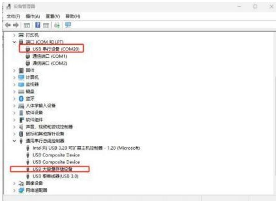
Figure 8 Device Recognized as USB Flash Drive Device/COM Port
