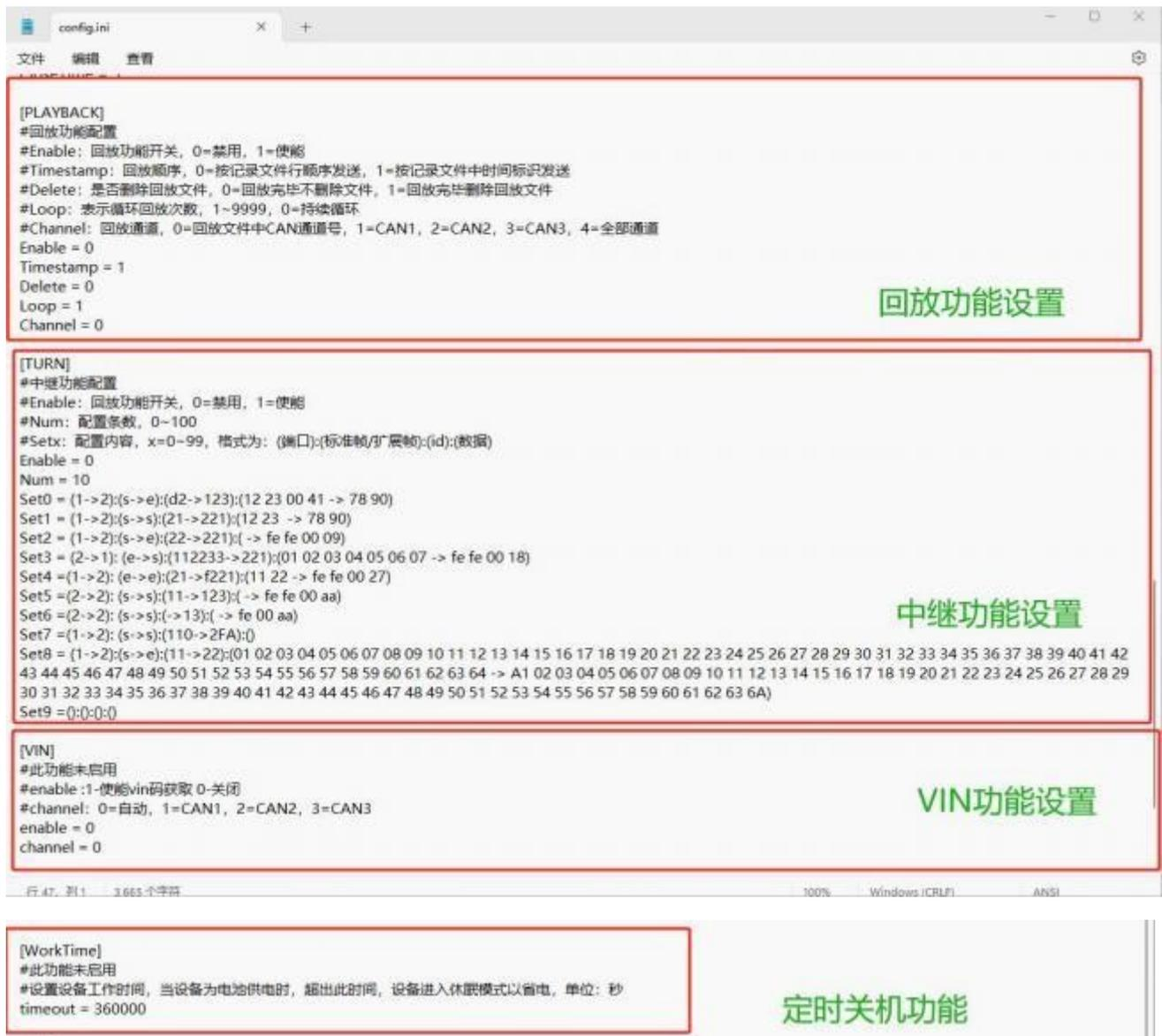
Figure 9 Example of Logger Profile InformationCAN
